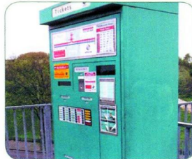
Grade 1.4003/410, painted [15 years in service], SASSDA, UK
